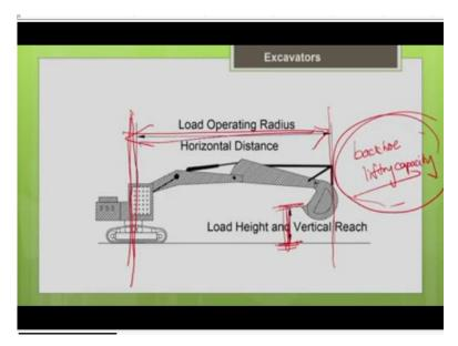
Another important thing you have to note that whenever the manufacturer provided you the lifting capacity for the backhoe. So, when they provide the lifting capacity for the backhoe they will give you a complete chart. So, this is because this also belongs to the cranes family. So, all these operations that are somewhat similar to the crane. So, you can see that based upon the operating radius, the lifting capacity of the machine will vary, what is the operating radius.
