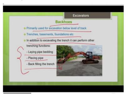
So, now let us discuss about the backhoes. So, you can see that the basic parts and operation are similar for both the machines but only thing to be noted is the digging motion of the bucket is in downward direction. So, it is preferred for the deep digging below the ground level, this machine is used for the digging below the ground level. So, mainly used for excavation below the level of track.
