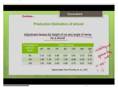
Now, let us see what are all the adjustment factors, we have to apply while doing the productivity estimation based upon the height of the cut of material actual height of cut of material in your project site and based upon the angle of swing that is going to depend upon the position of your truck relative to the position of your excavator. So, adjustment factors for the height of cut and the angle of swing for the shovel.
