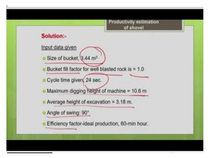
Let us see oh it is now that. So, in this slide, I have just summarized the data whatever the input data given in this problem. So, the size of bucket is 3.44 meter cube, that means it is a heaped bucket capacity given by the manufacturer, bucket fill factor is given us 1 for the well blasted rock, cycle time is given to you as 24 seconds, the maximum digging height for the machine is 10.6 meter.
