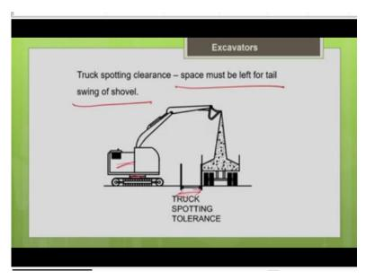
Another thing to be noted is truck spotting clearance. That means, as I told you, it is preferable to place a truck closer to the excavator. But at the same time, note that there should be some space left for the tail swing of the shovel. That means now you can have a complete 360 degree swing, you have a slewing ring here, you can have a complete 360 degree rotation about the mounting.
