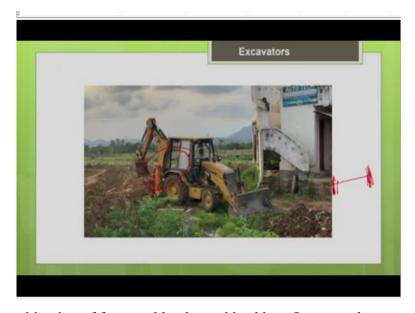
So, this is the combination of front end loader and backhoe. In some places you may need this combination because I may have to use a backhoe for excavating below the ground level, at the same time I may need a help of a front end loader to transport the material to a dumping position, when both are needed together then you have to go for this front end loader backhoe combination.
