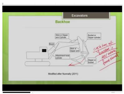
So, these are the basic operating parts of the backhoe it is similar to a front shovel only anything is digging motion of the bucket will be in downward direction. But one thing to note that cycle time of backhoe is 20% more when compared to front shovel. The reason is say whenever the
