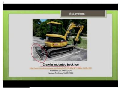
So, this is a crawler mounted backhoe a smaller one. So, let us different models are available. So, when you are working in a narrow space or confined areas you can go for a smaller size backhoe. So, it also has an attachment of the grader you can see for grading.
