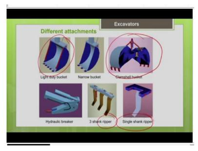
And use it for different applications. So, I can go for a light duty bucket. That means if you are going to handle lighter material, I can go for a wider bucket, but if you are going to handle harder material or denser materials, you go for a narrow bucket with a short tip radius. So, that we facilitate the digging operation. So, another attachment you can see clamshell bucket. So, this is also very commonly the mounted on excavators or it can be even mounted on the cranes.
