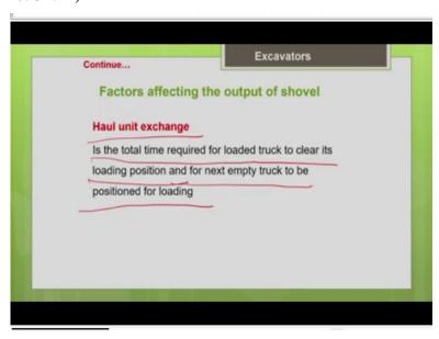
Other important factor is haul unit exchange time. That means the time needed for the loaded truck to leave its position. And for a new truck that is an empty truck to take the position. That
