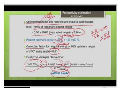
Now, as we discussed earlier, we have to find the optimum height for the machine, it is nothing but 50% of maximum digging height. I hope you know why we do to 50% because it is handling blasted rock, rock is a harder material to handle. So, take 50% of the maximum digging height. So, 0.5 into 10.6 meter it gives you 5.3 meter is the optimum height for the machine, but what is the actual height of cut it is dealing with it is 3.18 meter.
